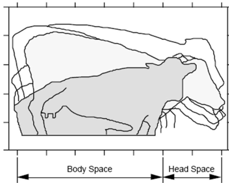
**Figure 2.** Forward lunge space is often blocked by walls or boards placed in front of the cows' resting space.
