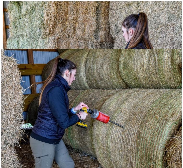
Figure 3. Round bales should be cored from the side to a depth of 15 to 18 inches.
