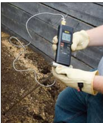
Figure 4. Example of an electronic thermometer. Note the temperature reading of 151°F.
