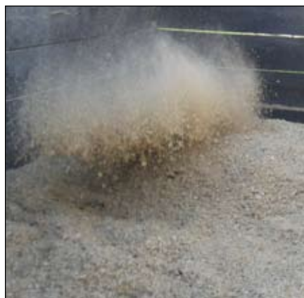
Figure 2. Wood chips being used as a bulking agent and carbon source.
