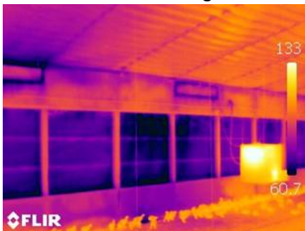
Figure 1.19 – Thermal images – leaky versus well insulated tunnel inlets
