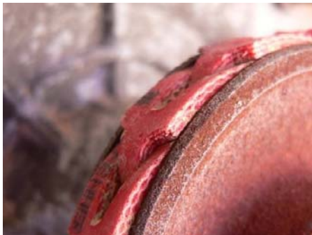
Figure 1.36 – Comparing new versus worn fan belts
