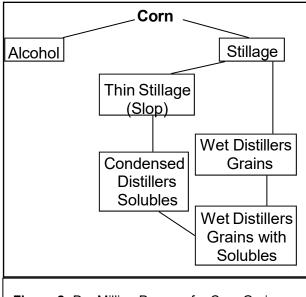
**Figure 2:** Dry Milling Process for Corn Grain (Source: Iowa State University - IBC-18 Extension Publication)
