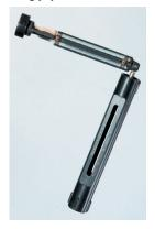
bulb temperatures to be used to reliably and accurately determine relative humidity. A sliding scale on the device allows the two temperatures to match. An arrow will indicate the relative humidity on another part of the scale. Obviously, no recording method is possible. Costs for a typical instrument are in the \$45 to \$70 range.
