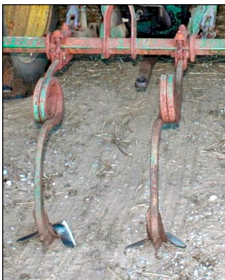
Figure 53. Sweeps or shovels may be added to tillage implement tines to provide more effective stirring. This is a cheap, effective addition to existing implements.
