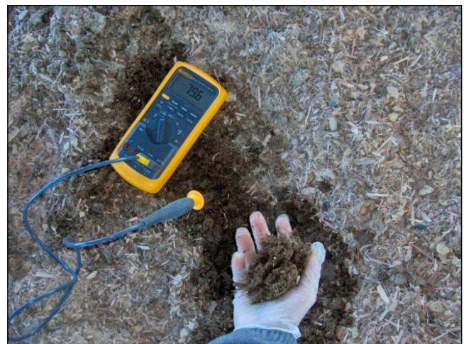
C. Example of compost that is too dry with insufficient temperature.
