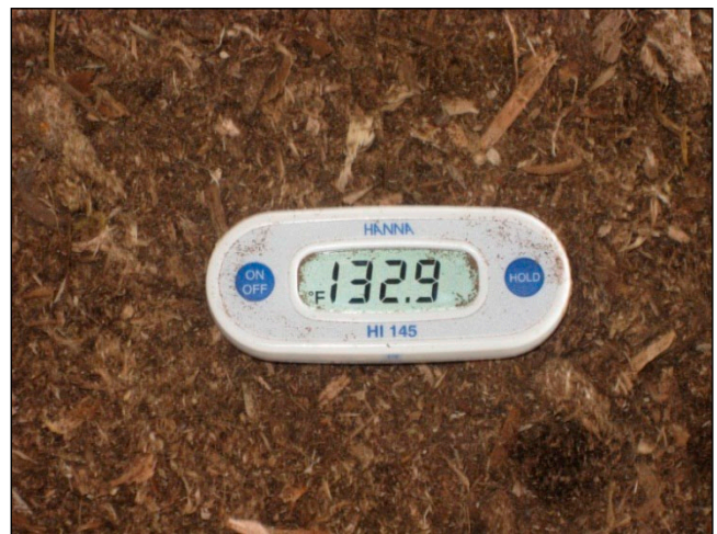
B. Example of compost heating well with high temperature and dry material.
