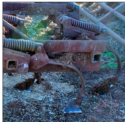
Figure 53. Sweeps or shovels may be added to tillage implement tines to provide more effective stirring. This is a cheap, effective addition to existing implements.
