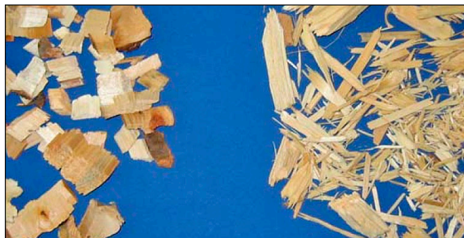
Figure 58. Wood chips produced with sharp blades (left) and blunt hammer (right).
